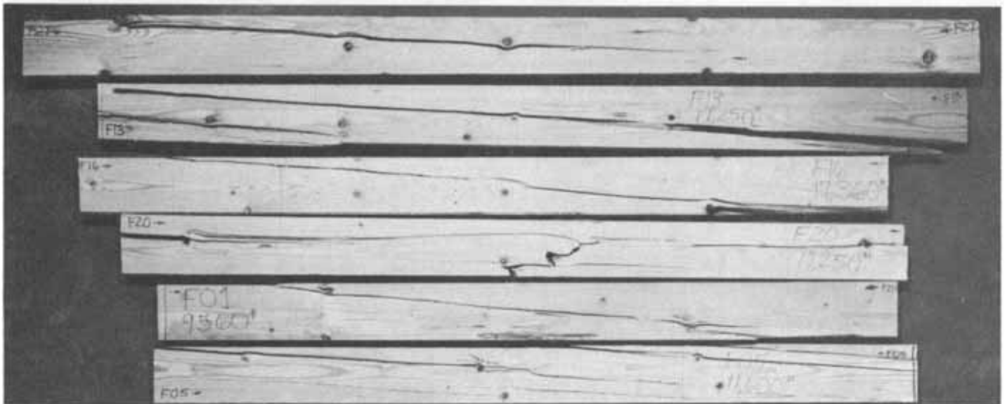
Figure A-B.—These 302-24 DF-L failures illustrate the typical, near-minimum quality of 302-24 tension lamina- tions selected. (M 147 136)
