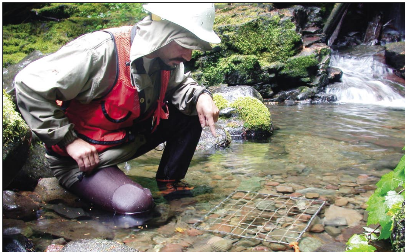
Figure 9—A sediment grid was used to quantify the percentage of fine sediments on the surface of pool tail substrate.
