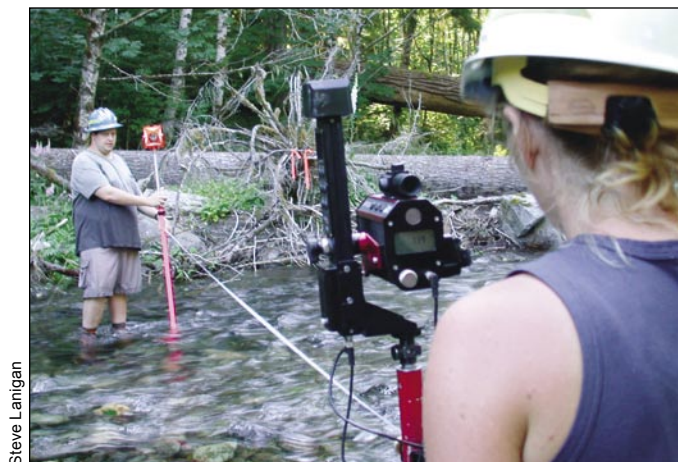
Figure 7—A laser level was used to measure cross-sectional profiles at transects placed throughout each stream reach. This information was then used to determine bankfull width-to-depth ratios and entrenchment ratios.
