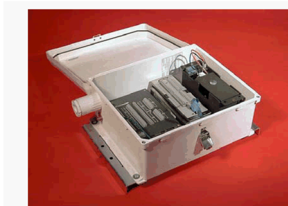
Figure 2 – Campbell-Scientific™ CR10X datalogger, mounted inside a weatherproof fiberglass enclosure, used to automatically collect and store data.
