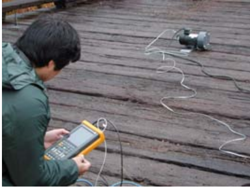
Figure 1. Forced vibration testing of field bridges with a forcing function.
