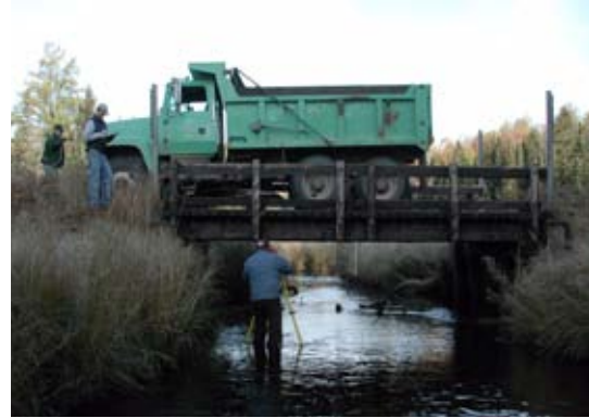
Figure 2. Static load testing of field bridges with a fully loaded gravel truck.
