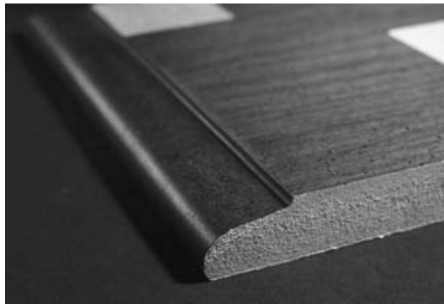
FIGURE 10.11 Thin veneer over medium-density fiberboard.
