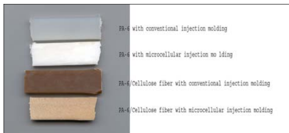
Figure 1 Sample color changes when microcellular injection molding process is used.
