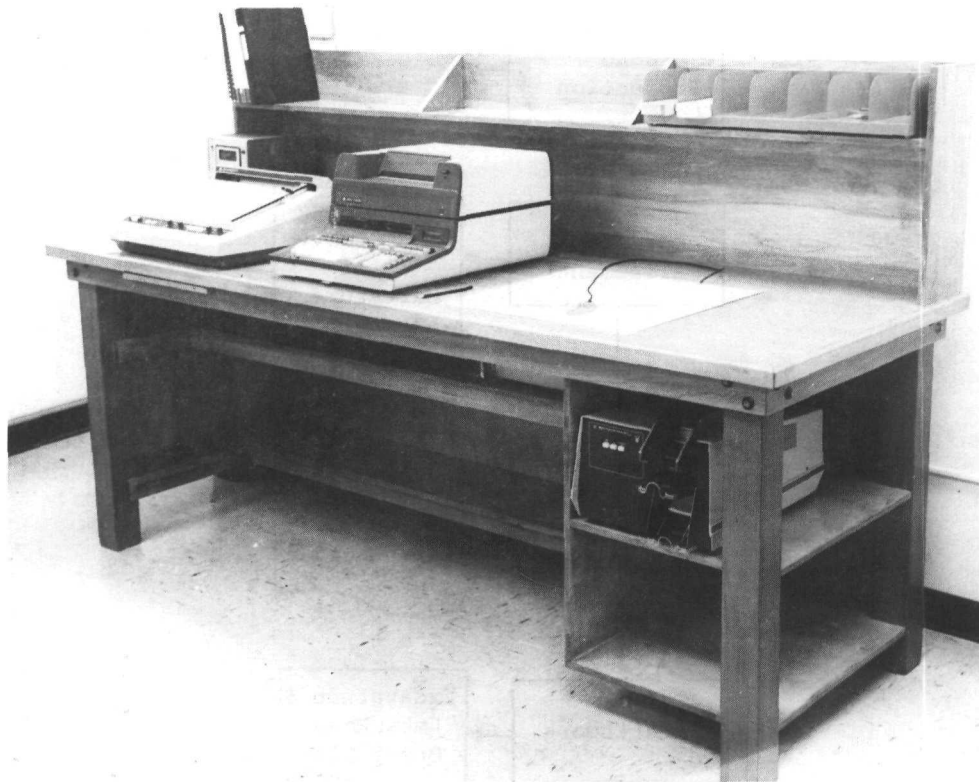
Figure 3.--Desk-top calculator system with digitizer, plotter, printer, and card reader.
