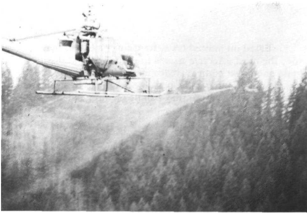
Figure 12.--If the Microfoil Boom ® is maintained in proper trim, the spray falls in a characteristic sheetlike pattern.
