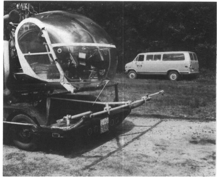
Figure 18.--A modified R-511 system with, five nozzles arranged on a short spray boom .
