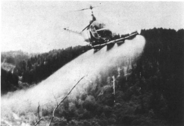
Figure 15.--Modified R-511 system applying Vistik-thickened sprays on the Siuslaw National Forest.
