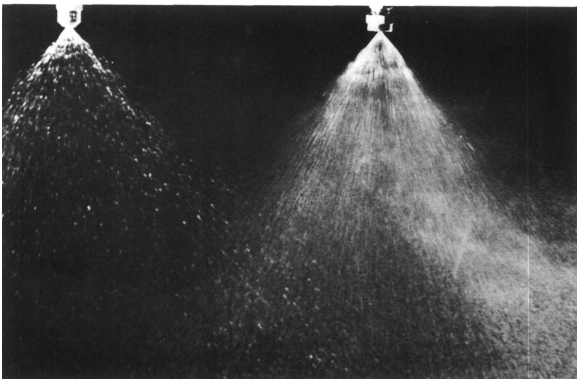
Figure 5.--Comparison of spray pattern from Raindrop ® (left) and hollow cone (right) nozzles (4m/h crosswind).
