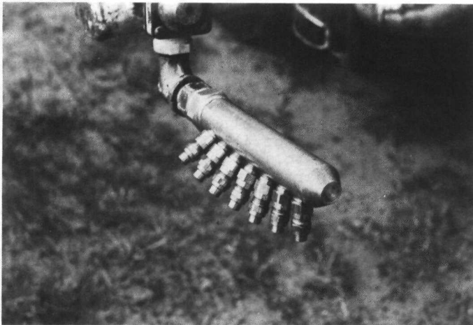
Figure 17.--A boomless sprayer uses cylinder manifolds mounted on the helicopter skid toes.
