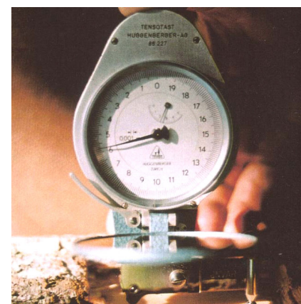
Figure 3.—Huggenberger tensotast (accurate to 0.001mm) used to measure growth stress. It is the movement of the two Phillips head screws (bottom) which is measured after the wood is cut free on each side. The instrument is provided with calibration bars.
