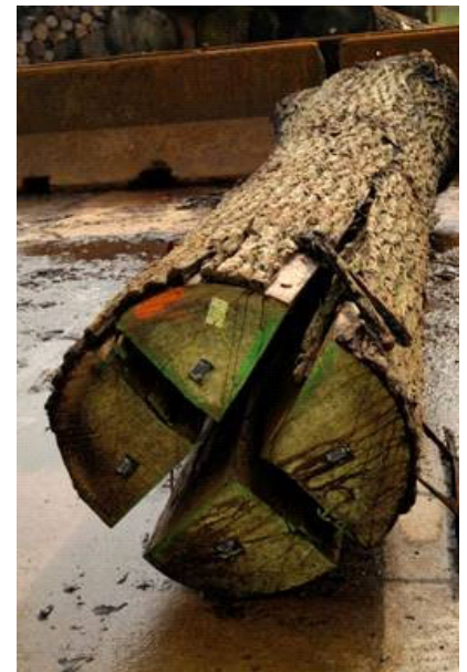
Figure 1.—High quality walnut veneer log which has been severely degraded due to the release of growth stress.
