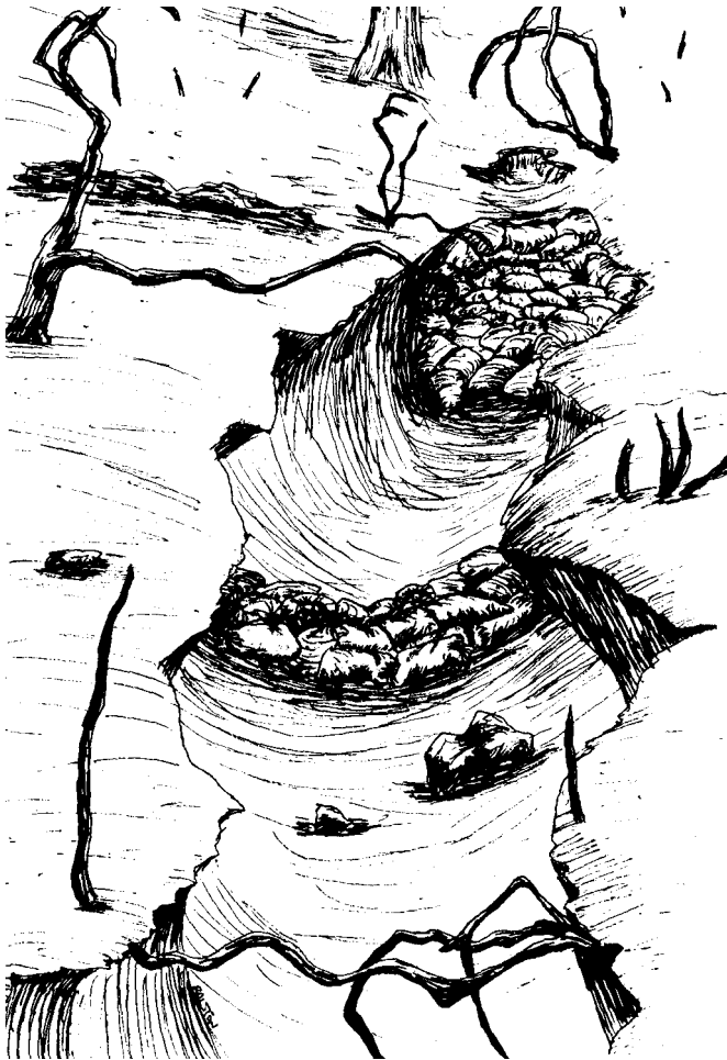
Figure 2--Sand bag check dam. Rot-proof sand bags are filled on-site and keyed to gully bottom and walls.
