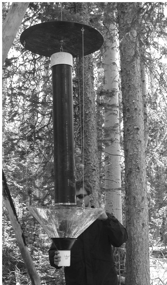
Fig. 2. View of the bark-baited pipe trap. Piping is 20-cm-diameter ABS, topped with a PVC cap with two 5-cm attic vents. Additional ventilation is provided by hundreds of 2-mm holes drilled into the pipe surface and by window screening held onto the pipe bottom with a hose clamp. The lure for the trap is composed of six female-infested bark sections suspended within the pipe.
