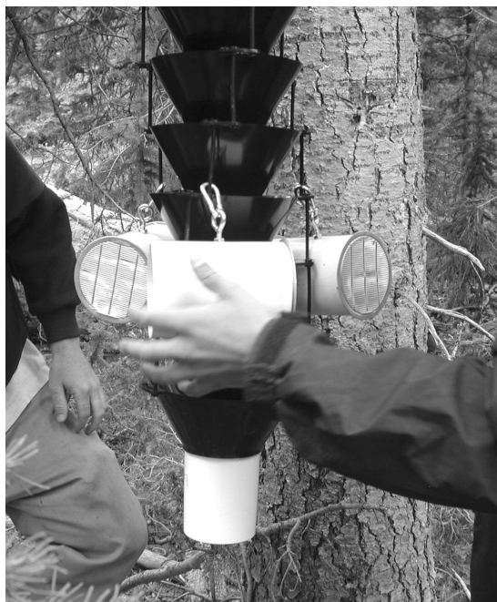
Fig. 3. View of the bark-baited funnel trap. Trap is a commercially available 16-unit funnel trap (ChemTica International). Female-infested bark sections are held individually in each of three vented PVC sections.
