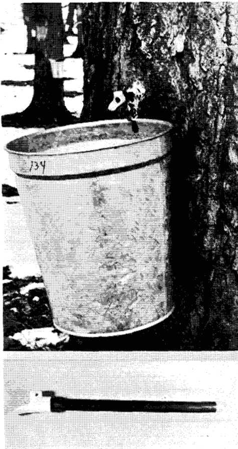
Figure 1.—For collecting sap flow from taphole depths greater than 1 inch, copper tubes were inserted into the taphole to stop the flow from lesser depths. Inset below shows the copper tube, fitted with a plastic spout.
