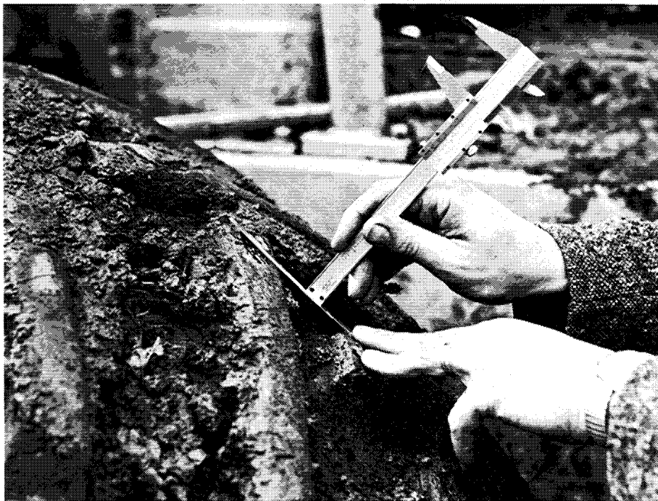
Figure 2.—The method used to measure depth of tread.
