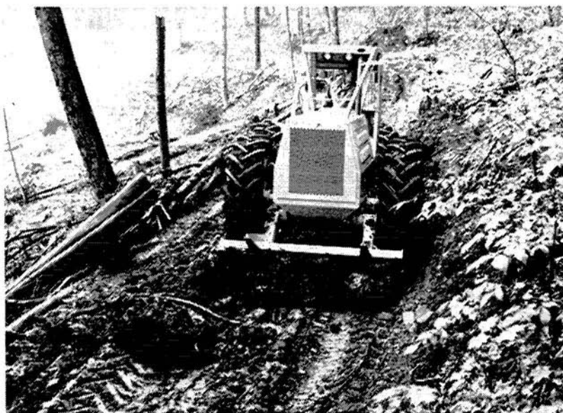
Figure 6.—Scraping this skidroad during spare time kept ruts from forming and increased the traction for winching and skidding.
