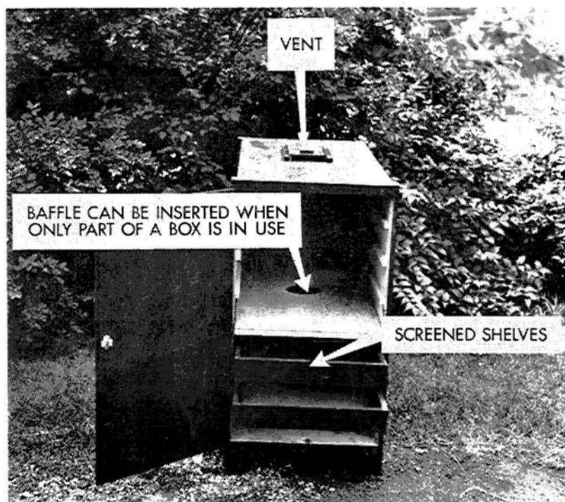
Figure 10.—Side (above) and front (below) views of a simple drying box, using a forced-air electric space heater.
