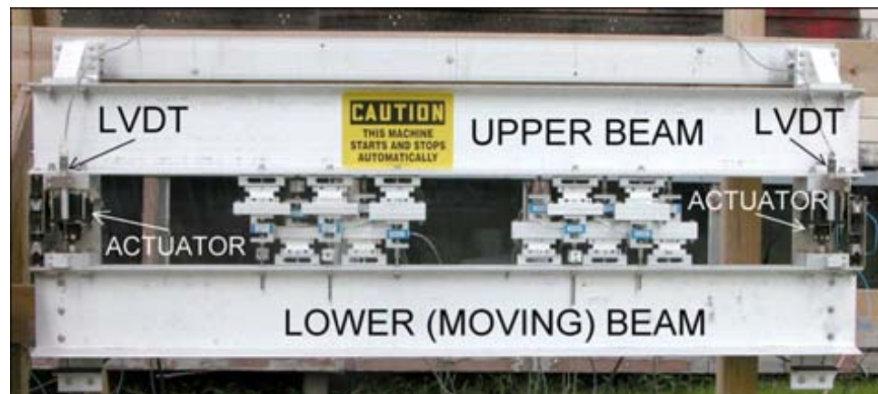
Figure 4. The CFTA type outdoor exposure apparatus.
