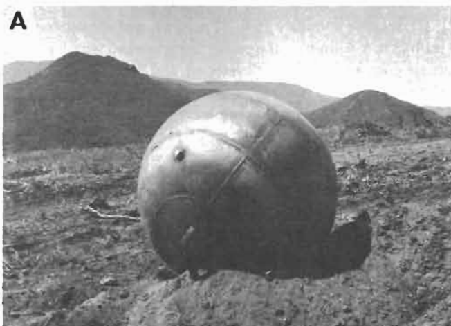
Figure 24 —To crush chaparral shrubs, a Navy buoy, or ball (A) is filled with water, attached to a tractor by a chain, and dragged along
