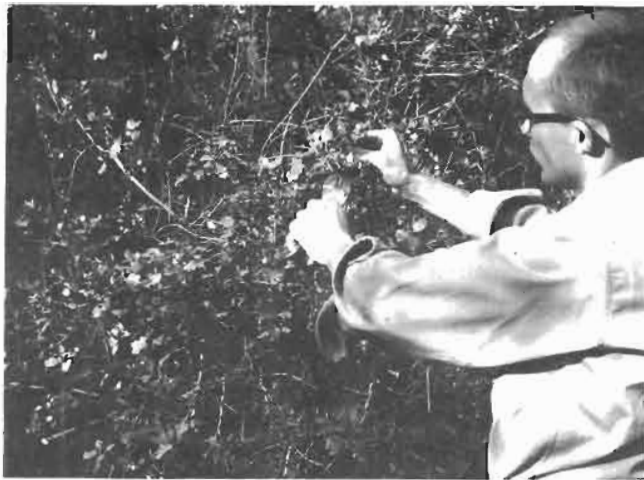
Figure 7 —Live fuel moisture is calculated using fresh and oven-dry weights of twigs clipped to ½ inch diameter.
