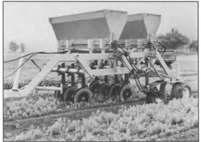
Figure 42 —Machine used to band granular ammonium phosphate sulfate (NPS) fertilizer between rows of newly emerged seedlings, second-year seedlings, and transplanted 1-0 seedlings in Humboldt Nursery. Granules of NPS are fed from the hoppers to the bed by a bank of flexible hoses mounted behind two gangs of paired colters. The colters are set to cut soil channels 1 inch (2.5 cm) deep.
