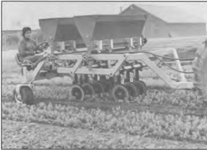
Figure 42 —Machine used to band granular ammonium phosphate sulfate (NPS) fertilizer between rows of newly emerged seedlings, second-year seedlings, and transplanted 1-0 seedlings in Humboldt Nursery. Granules of NPS are fed from the hoppers to the bed by a bank of flexible hoses mounted behind two gangs of paired colters. The colters are set to cut soil channels 1 inch (2.5 cm) deep.
