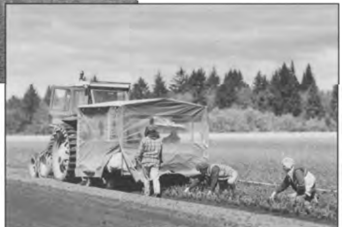
Figure 43 —Machine used to transplant seedlings for 1-1 planting stock in Humboldt Nursery. The 1-0 seedlings are root-pruned 5 inches (13 cm) below the cotyledons just after lifting, held in cold storage, and transplanted into six rows per bed. Transplanting results in a bed density of 6 to 8 stems per square foot (65 to 86 stems per m 2 ).
