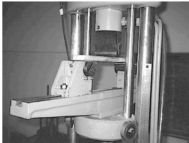
Fig. 2 MOR and MOE test set-up (Losenhausen test machine)
