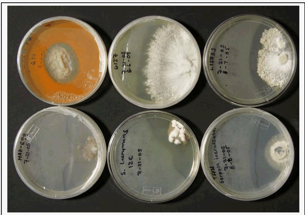
Figure 2: Growth of 4 Fungal Strains on 0.1% NHA treated MEA Plates Top row: MAD 497, TYP 4137, TYP-L-15755 Bottom row: MAD 498, S. lacrymans 12C, TFFH S. lacrymans
