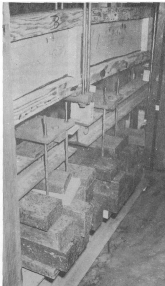
Figure 4. — Six-foot I-beams in cyclic humidity environment. (M 142 284)
