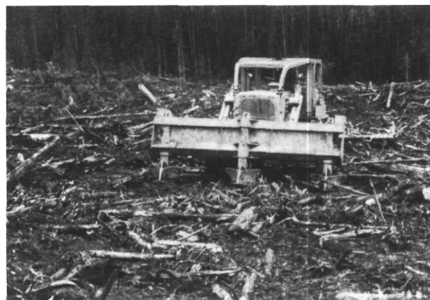
Toothed blade. A companion to the anchor chain drag.
