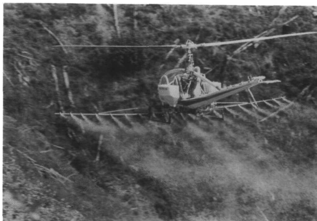
Figure 9.—Aerial application of an oil-in-water emulsion of 2,4,5-T as a foam spray during critical weather conditions: wind velocity about 5 m.p.h. and relative humidity near 50 percent. Note absence of whorls evident in figure 1.
