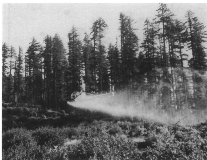
Figure 1.—Fine droplets may be lifted high above the helicopter in large whorls from the end of conventional booms. These fine droplets can drift with the wind or evaporate and drift in vapor form.
