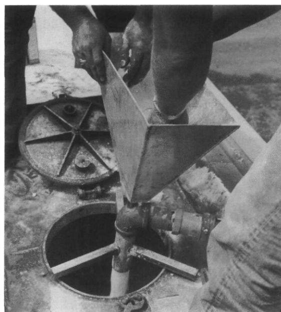
Figure 6.—A funnel for adding and dispersing Vistik in the nurse tank by feeding the powder into a 2-inch bypass.
