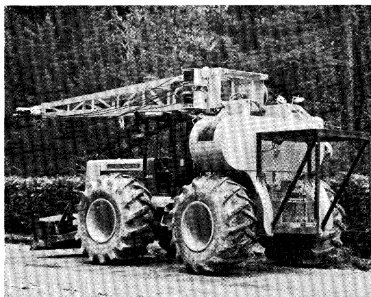
Figure 3.--Prototype peewee yarder with tower lowered.
