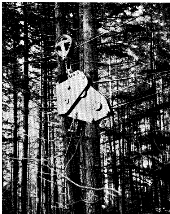
Figure 4.--Slack-pulling carriage designed by the Forest Engineering Research Unit.
