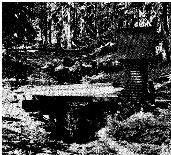
Figure 3.--Typical streamflow measuring section.
