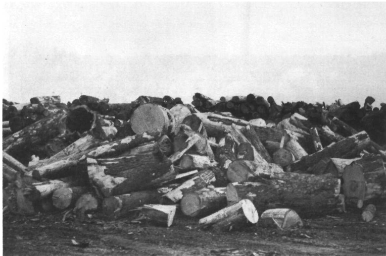
Figure 8.--Broken ends, swelled butts, etc., can be split and barked in a drum barker.
