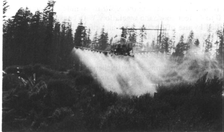
Figure 5.—To reduce drift and evaporation and insure accurate application of herbicidal sprays, helicopters fly at minimum safe flying height over brushfields.
