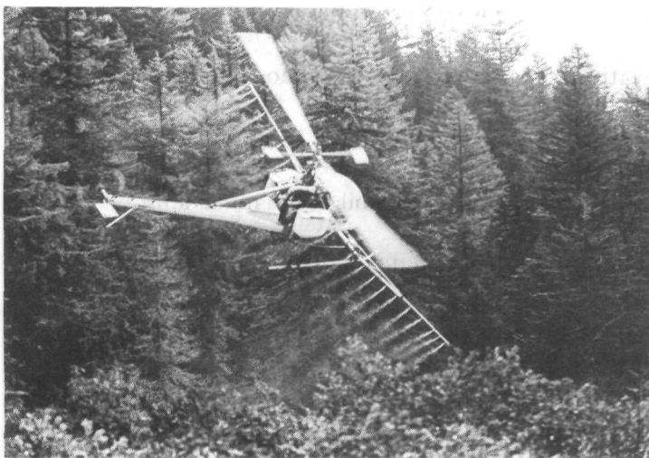
Figure 8.—Helicopter applying 5 gallons of herbicidal spray per acre; the second 5 gallons per acre will be applied at right angles to the initial lines of flight.
