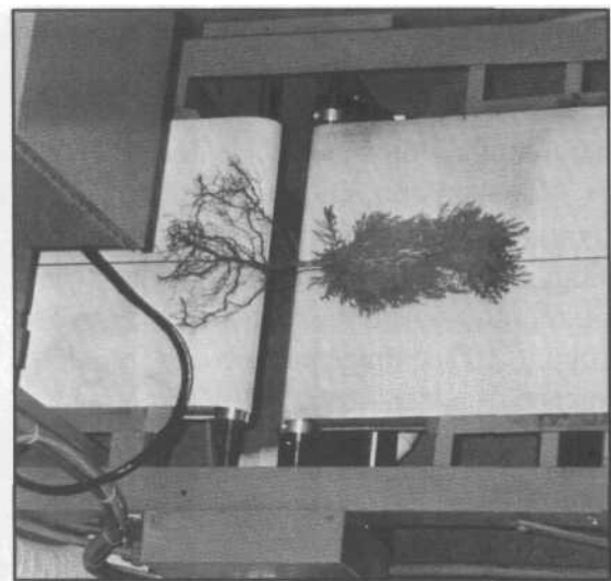
Figure 5. Machine vision quality control inspection station for tree seedlings.
