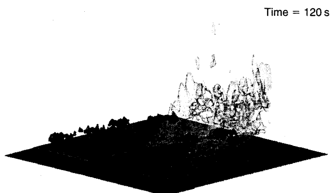
Fig. 6. Image from the patches, less ground fuel (PLGF) simulation 120 s after ignition. The colors on the horizontal plane indicate bulk ground fuel density, with black being no fuel and brown being short grass and litter. The dark green isosurfaces show the tree locations, and the black isosurfaces show parts of the canopy that have been significantly burned. The orange, red, and grey isosurfaces indicate regions of hot gases.
