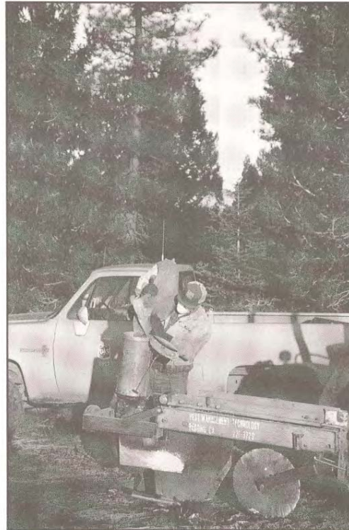
Figure 10—Loading bait into a heavy-duty burrow builder modified for forest use (Photo by Warren Sauer)
