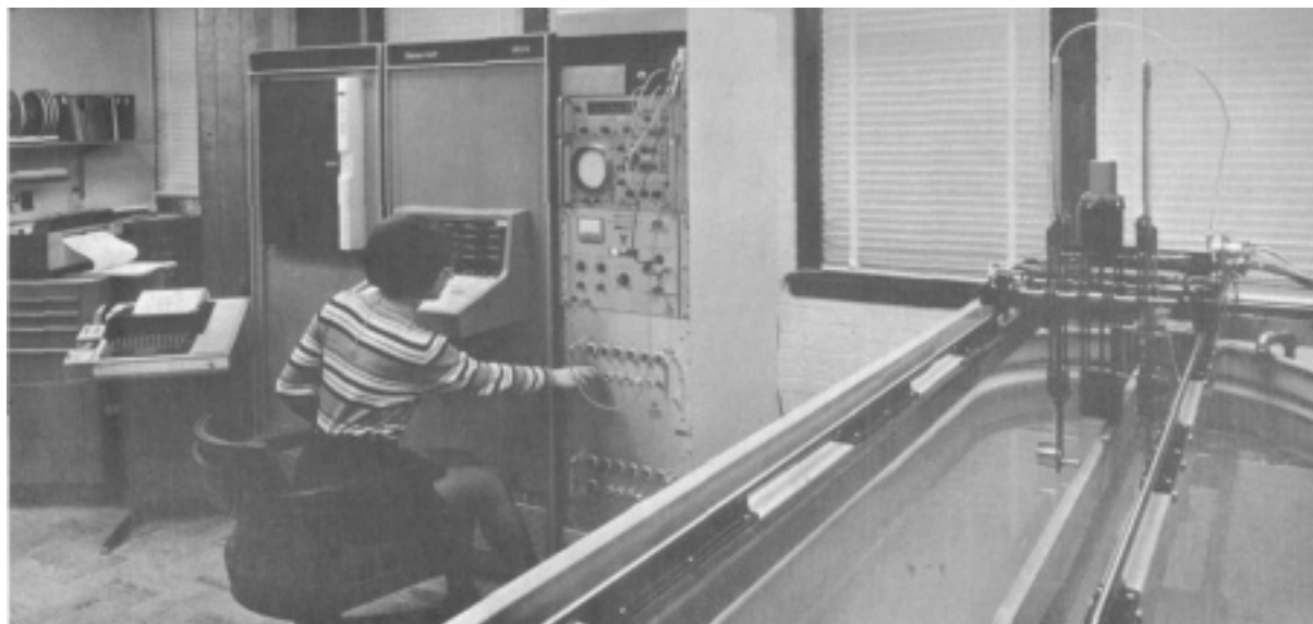
Figure 11.—The computer-controlled lumber scanning system for laboratory evaluation of ultrasonic lumber defect detection.
