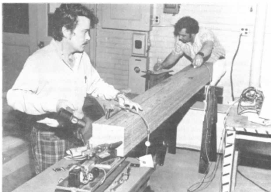
Figure 14.—Stress-wave measurement on an 8-foot-veneer tie.
