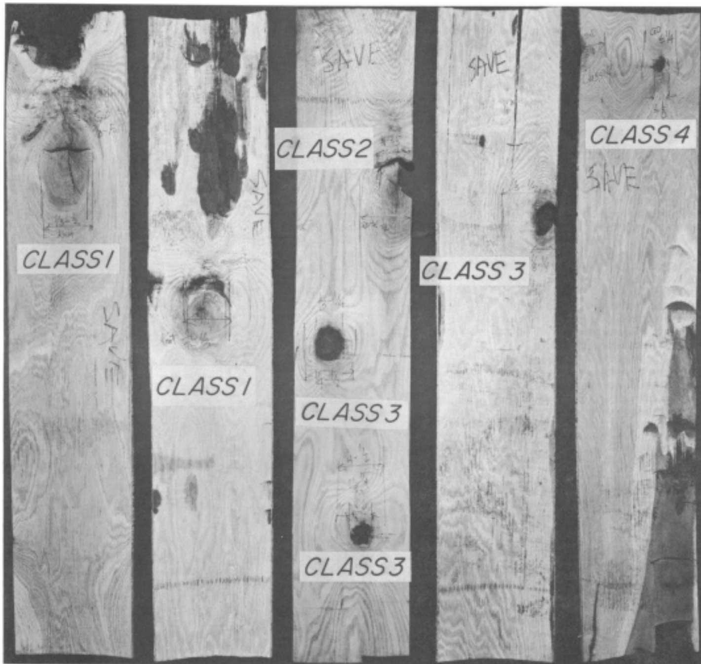
Figure 3.—Classification of knots in typical 10-inch-wide by 4-foot-long red oak veneer. Knot diameter and grain deviation expressed as a fraction of veneer width. The veneer shown was not used in ties because of wane.
