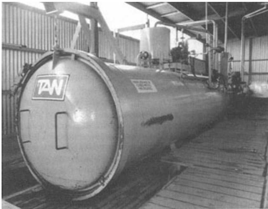
Figure 9.4. CCA pressure treatment plant. The chemical storage tanks are out of sight.
