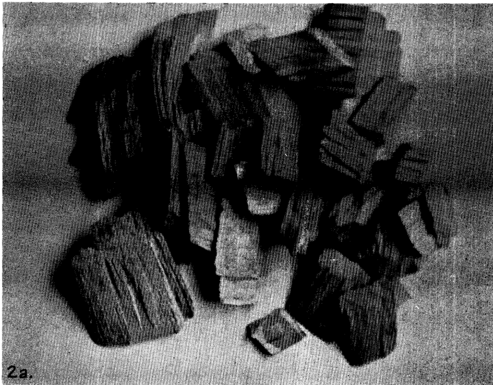
Figure 2a.--Alder chips (natural size) at start of test, no decay.
