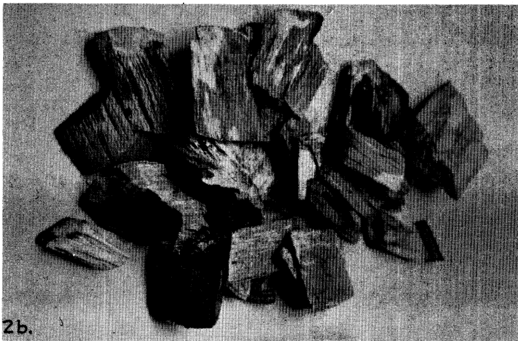
Figure 2b.--Alder chips showing decay after one year in 100 percent alder pile.
