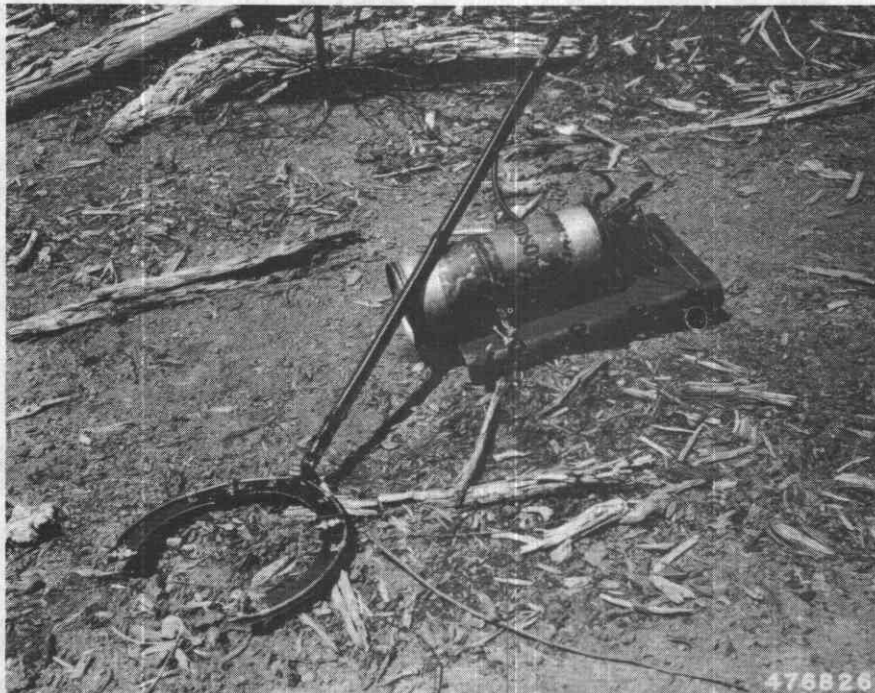
Figure 1.--Equipment used for basal treatment to kill red alder. (F.S. Photo 476826)
