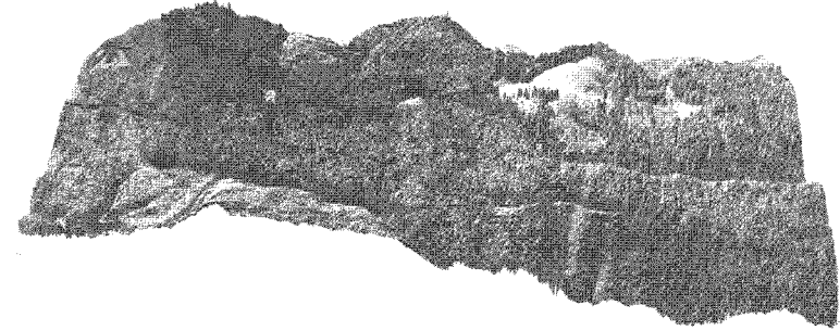
Figure 3-11. Shaded relief of the canopy surface model generated from X-band IFSAR data at Capitol Forest study area, Washington, USA. (See also color plate 3-11 on p. CP5)
