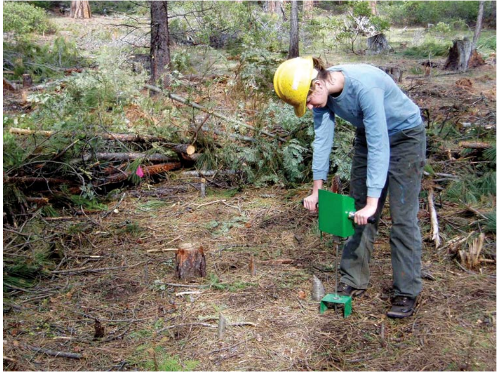
Measuring soil resistance using the recording soil penetrometer.
