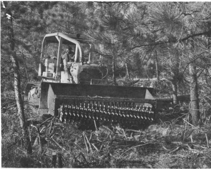
Figure 7.—A "Tomahawk" mounted on a D-6 crawler tractor. This attachment weighs approximately 2,700 pounds and is useful for crushing slash and brush.
