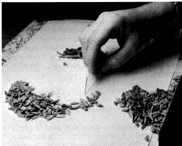
Figure 6. —In a purity analysis, the working sample is divided into component parts—pure seed, other crop seed, weed seed, and inert matter.
