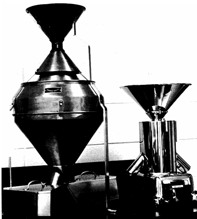
Figure 5. —Mechanical dividers can be used to sample a small lot or to split an oversize sample.
