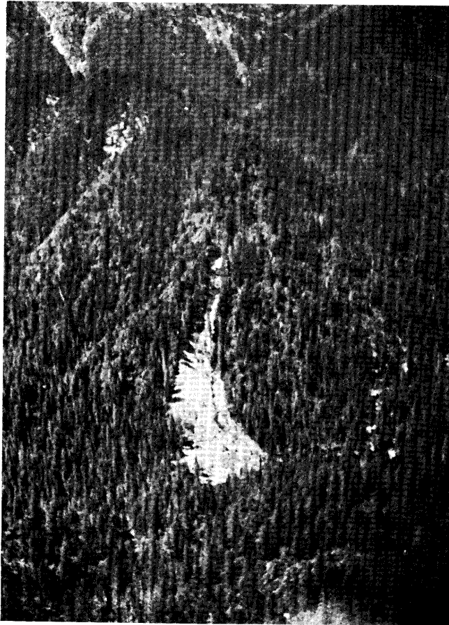
Figure 4.--Debris avalanche resulting from a road prism failure.
