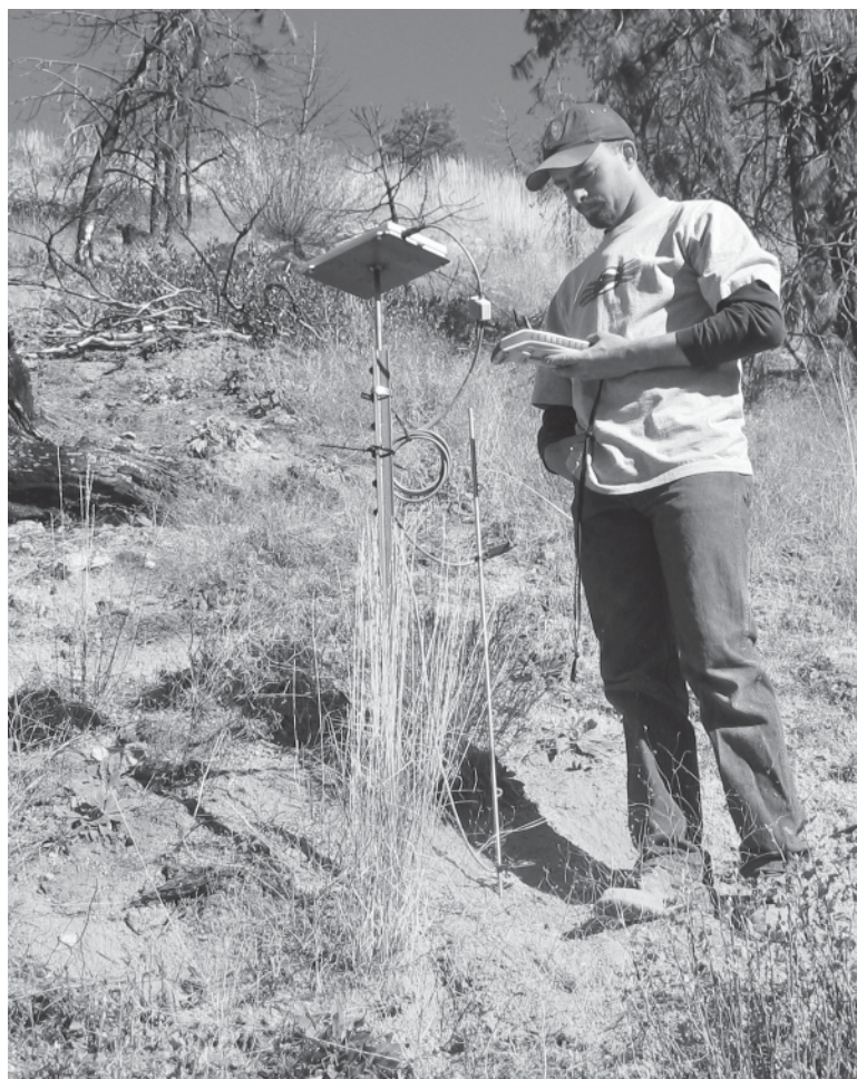
Figure 1 —AXTracker satellite transmitters can be used to monitor remote conditions such as temperature, facility intrusions, or track vehicles if coupled with GPS.
