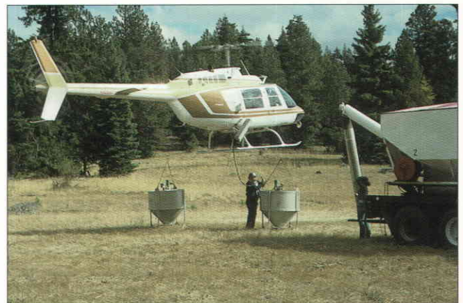
Color plate D—Helicopter preparing to lift loaded bucket used for applying fertilizer to experimental plots.
