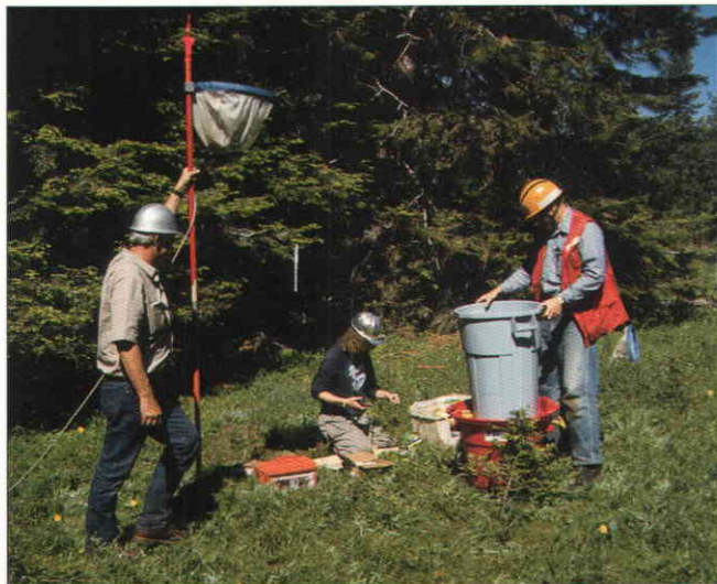
Color plate H—Processing foliage samples in the plot by beating clipped branches inside drum to remove arthropods from clipped branches.
