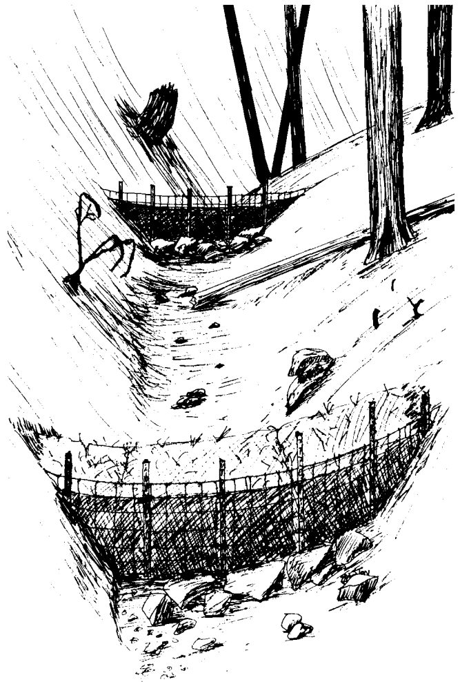
Figure 1--Straw bale check dam. Bales are wrapped in plastic netting, placed against woven wire fence, sealed at ground line, and staked.
