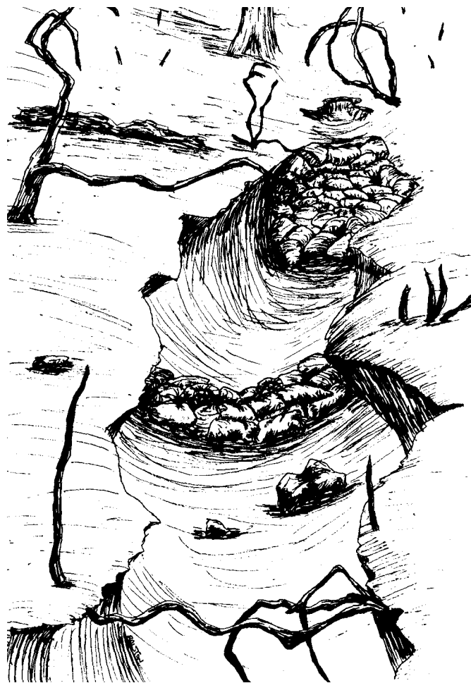
Figure 2--Sand bag check dam. Rot-proof sand bags are filled on-site and keyed to gully bottom and walls.
