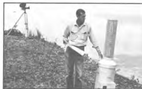
To investigate the basic processes of water yield from fog-drip in Hawaii, watershed researchers "milked" water from impinging clouds over Mount Kaala.
