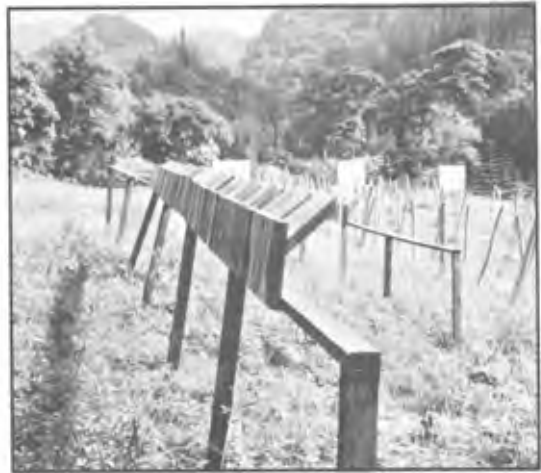
Wood products research included exposing samples of wood to the elements of weather, insects, and decay organisms.
