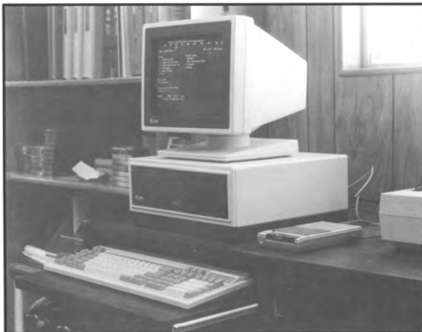
Figure 9 --Data collected by the datalogger and stored on the tape recorder are translated using an IBM-compatible computer.
