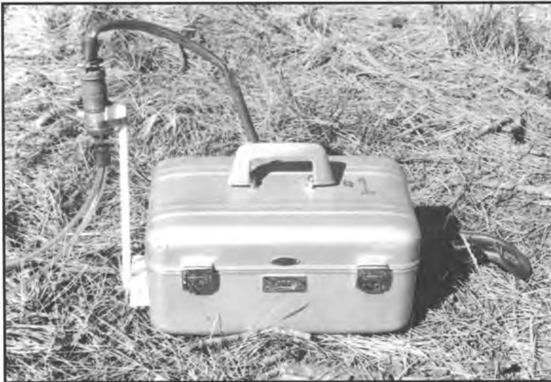
Figure 12 --Thermocouple wire socket connector is mounted on a field stand and attached to the pigtail and datalogger when measuring ambient soil temperature.
