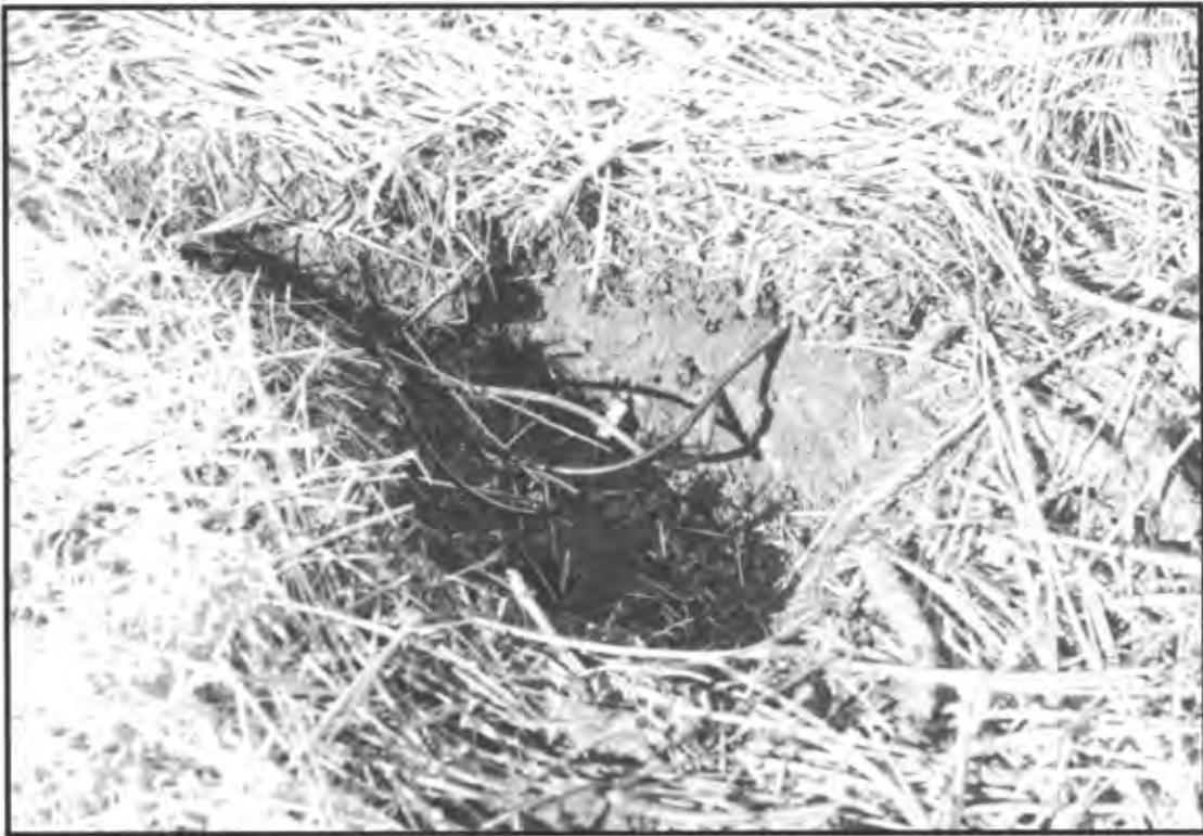
Figure 11 --Brass tube thermocouples are installed horizontally to measure ambient soil temperatures.
