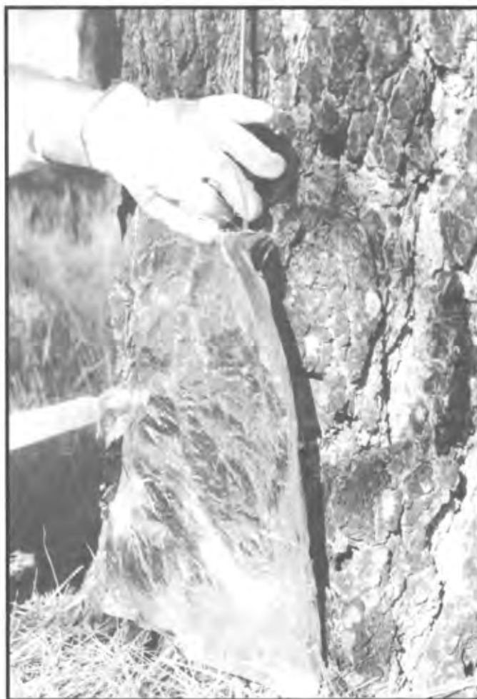
Figure 17--(e) Aluminized fabric and fiberglass insulation are attached to the tree with aluminum nails over the rectangular bark segment and thermocouple-extension wire connection.
