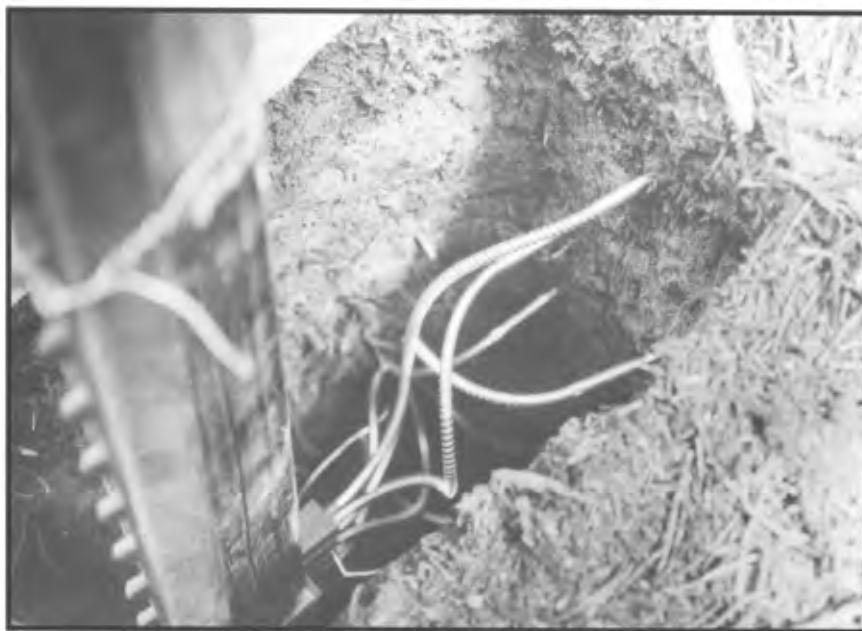
Figure 14 --Thermocouples are inserted horizontally into soil in a staggered configuration, and the portion of the extension cable protected by galvanized metal downspout is secured to a fence post.
