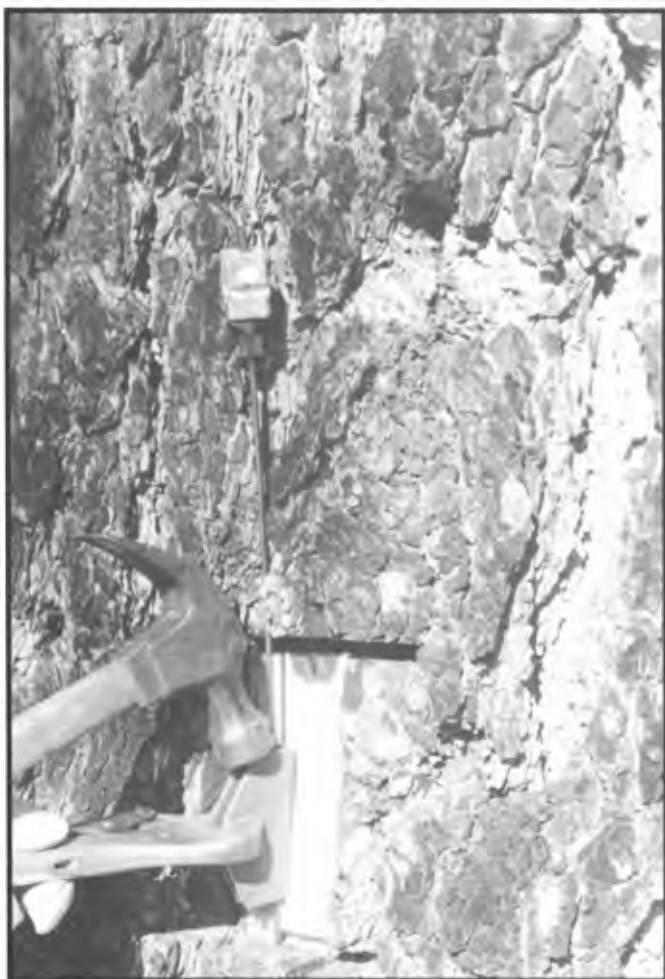
Figure 17--(d) With Visegrip applied, a hammer can be used to tap the thermocouple probe so that the tip is about halfway between the soil surface and the forest floor surface.
