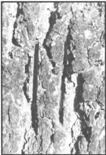
Figure 17-- Thermocouples are inserted into the cambium in a step-by-step procedure. (a) Two vertical cuts are made in the bark with a chain saw.
