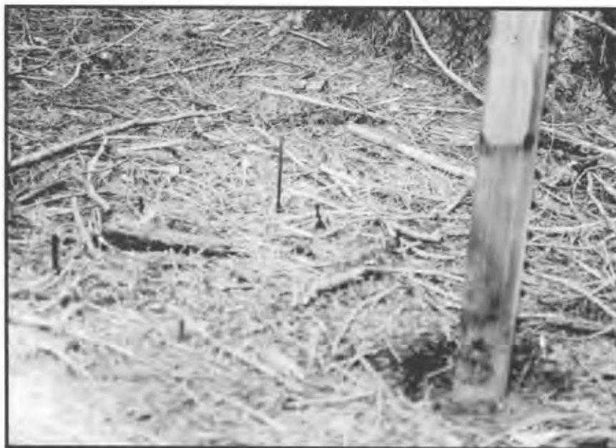
Figure 15 --Completed soil temperature monitoring site should resemble natural conditions.
