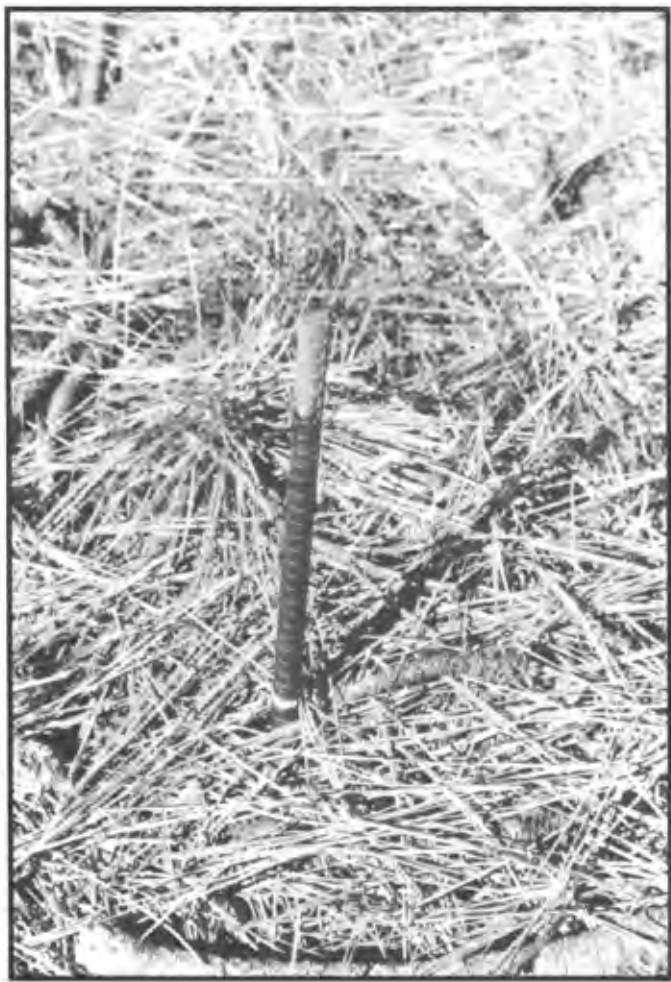
Figure 16 --Notched concrete reinforcing rods measure depth of the forest floor to determine the amount consumed by fire.
