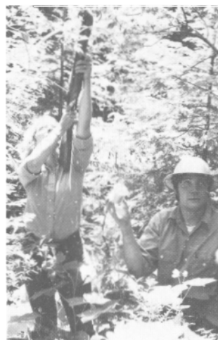
Figure 13 —Fluorescent streamers can be positioned in the tops of trees by using crossbows (A) or signal guns (B) to shoot lines with attached streamers over the trees.
