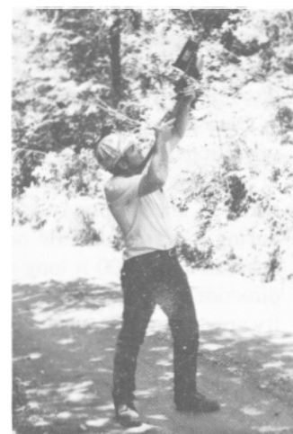
Figure 13 —Fluorescent streamers can be positioned in the tops of trees by using crossbows (A) or signal guns (B) to shoot lines with attached streamers over the trees.
