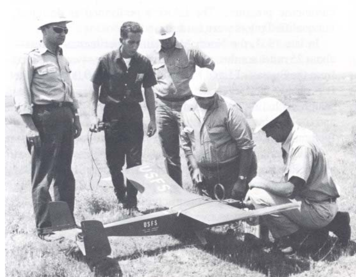
Figure 13 --The low altitude retrievable probe (LARP), a radio controlled drone airplane. The LARP was designed to fly in and around the smoke column of a fire gathering weather information.
