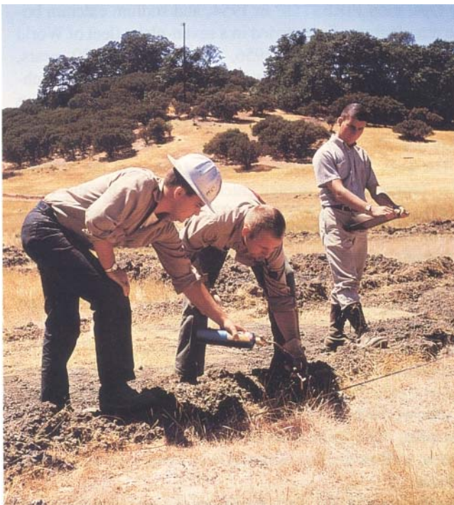
Figure 2 --Forest Fire Laboratory researchers attempting to ignite "weatherproof" fire retardant. The objective was to find a retardant that could be used to fire proof roadsides and around campgrounds for the duration of the fire season.
