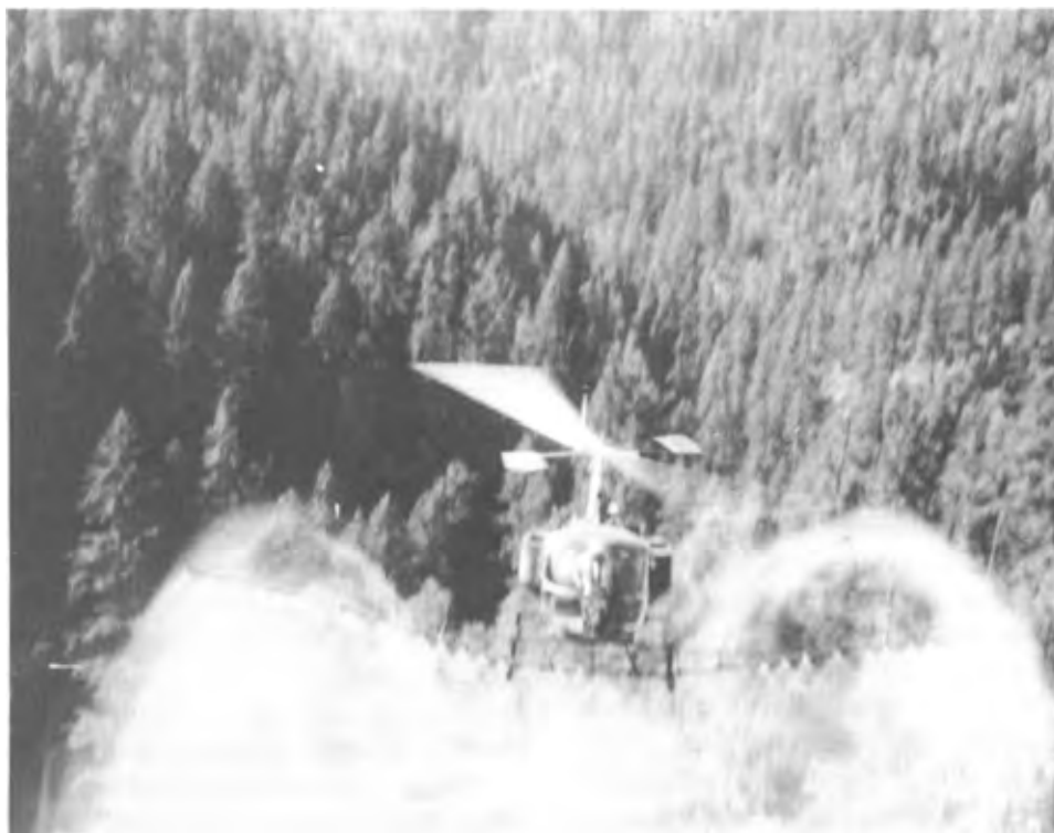
Figure 6 —On steep ground, herbicide application by helicopter is an economical and effective method of site preparation.
