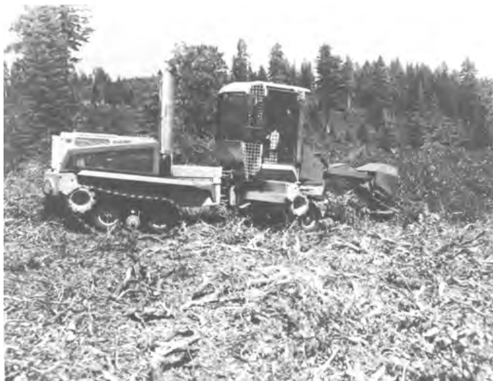
Figure 5 —Masticators are useful for "shortening" tall brush and leaving the ground covered with organic material.
