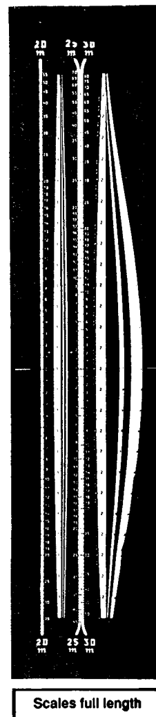
Figure 3-Relaskop scales, full length and as actually seen through viewfinder
