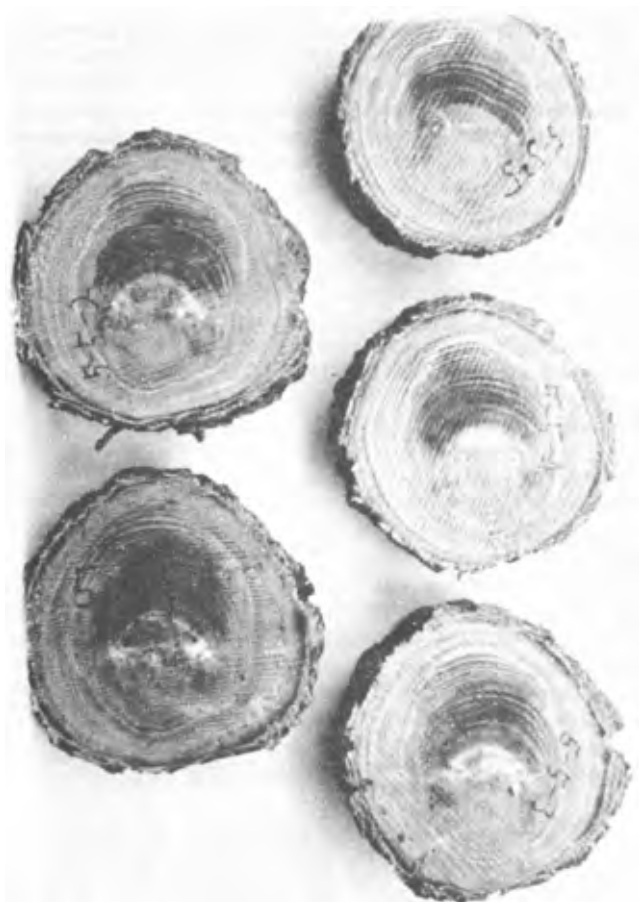
Figure 3 --Cross-section of white fir incubated for H. annosum . White conidiophores produced around decay column.
